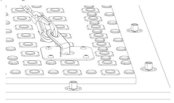
With the help of the chain sling, the panel can be moved to the desired position and installed.
