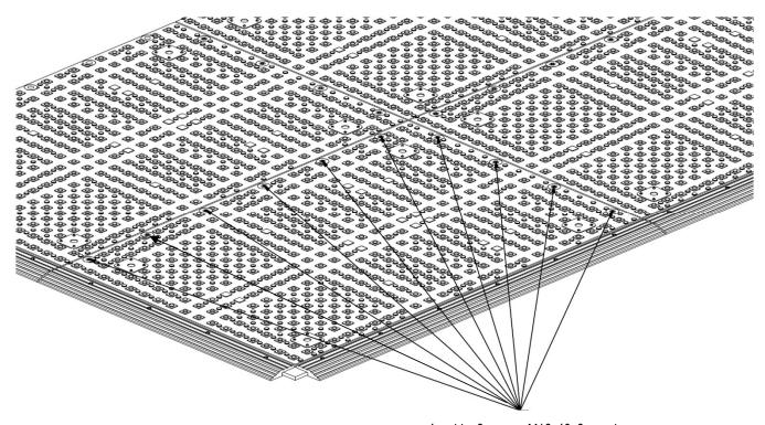
4m side: 8x screw M16x40, 8x washer 2m side: 4x screw M16x40, 4x washer
